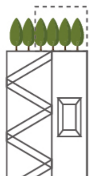
无机房电梯的机房 Machine room in machine roomless elevator
