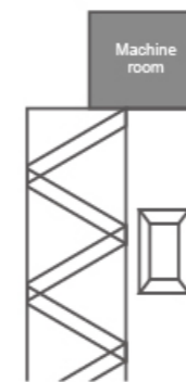
普通机房电梯的机房 Machine room in machine room elevator
